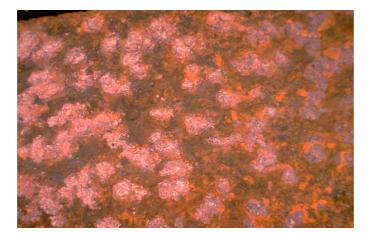
This rust grade is corresponding with rust grade D as described in SSPC-VIS 1. In this standard reference photographs illustrate four initial rust conditions before surface preparation, covering the range from intact mill scale to rusted and pitted steel. For tank bottom maintenance rust grades greater than B is mostly observed. Corroded tanks with a rust grade greater than B should have a surface pretreatment as is also mentioned in SSPC-VIS-1.
